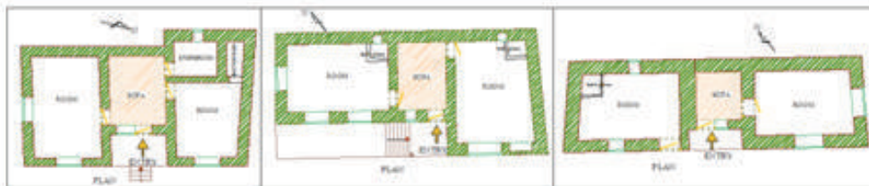
Fig. 13-9. Plan types implemented in the region with an anteroom in the middle.
