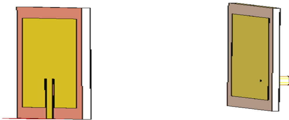
Figure 13. Sides of microstrip line feed and coaxial probe feed of MPAs
