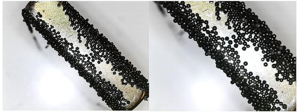
Fig. 1 Optical microscope view of interacting and self-assembling activated carbon spheres on a NdFeB magnet
