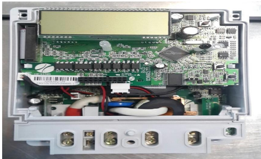
Figure 8 phase smart power measurement device [26]
