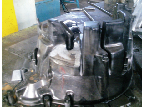
FIGURE 14: Fracture on the fix side of the die was produced with TOOLOX 44 (After 20,000 cycles' test).
