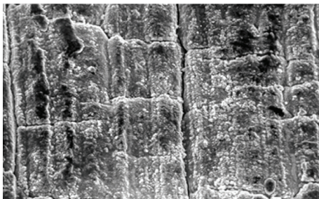
FIGURE 3: SEM microstructures of thermal fatigue cracks [1.2344 (H13)] [12].
