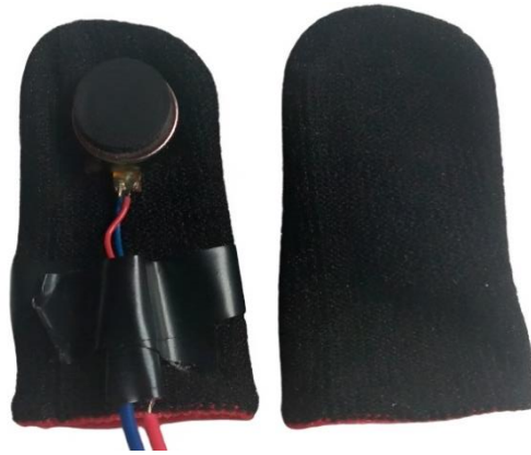
Figure 19. Haptic Fingertip Device (HFD) for Vibrotactile feedback
