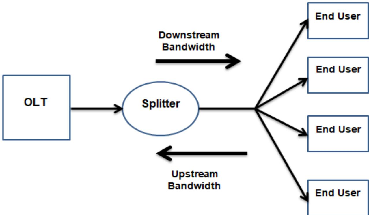
**Figure 2. 7:** Gigabit Passive Optical Network
