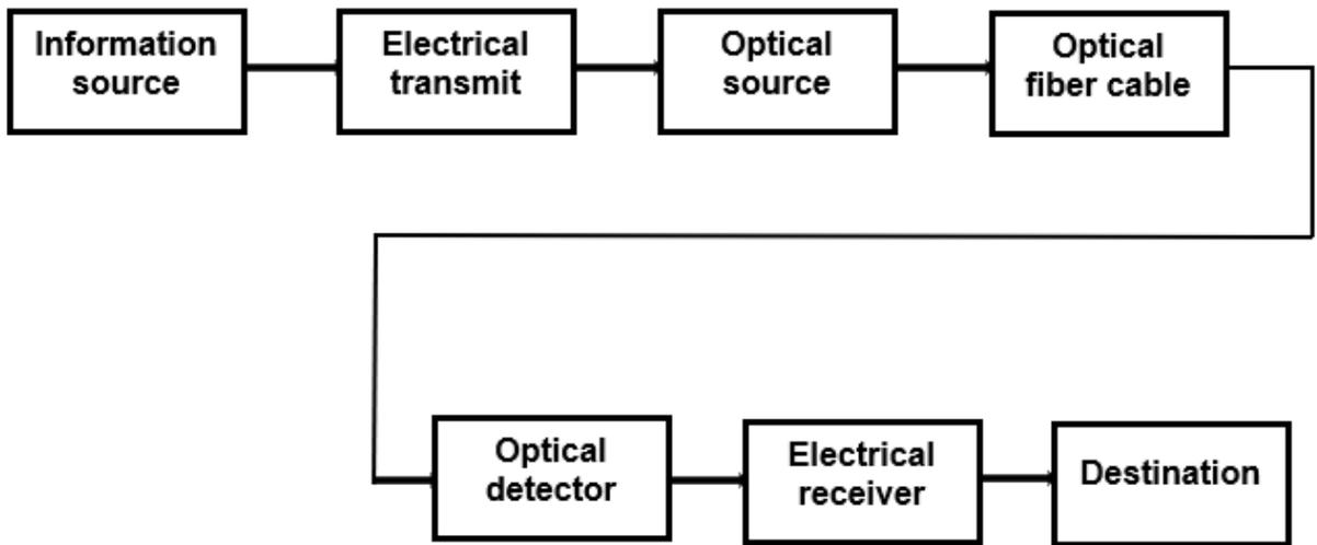
**Figure 2. 2:** Fiber Optic of Communication System
