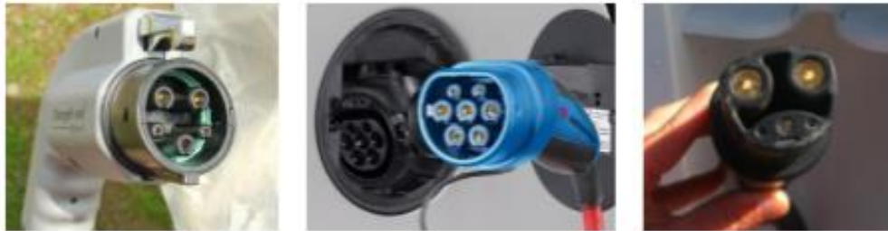
Figure 14 Plug for Ac charging- From left show module 1 used in US, in the middle module 1 used in European and in the right Tesla plug.
