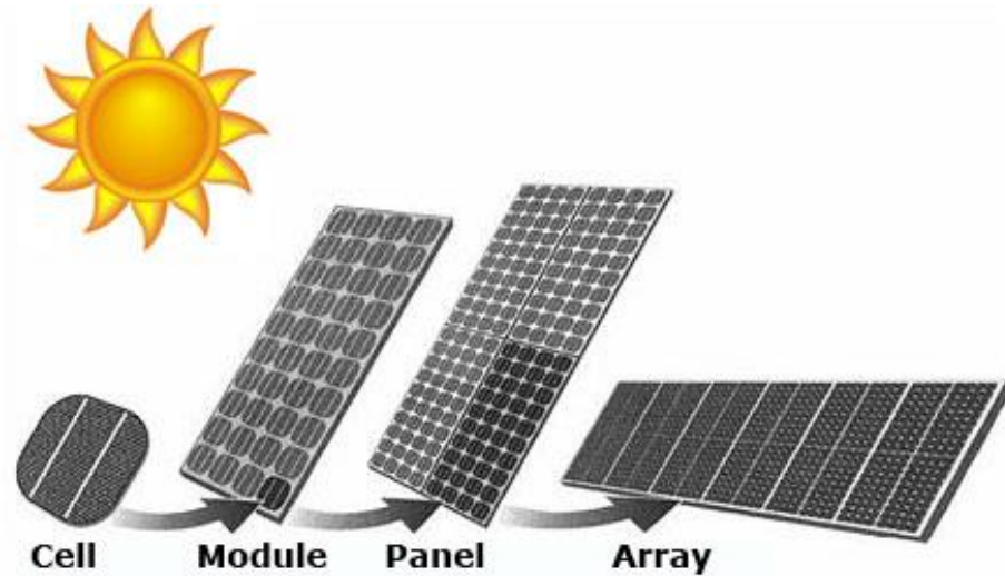
Figure 4 From cell to array.
