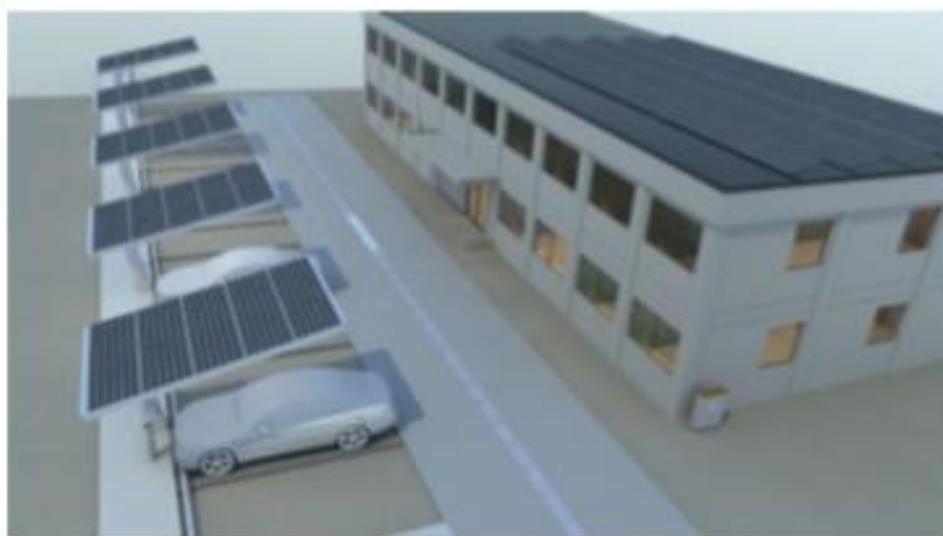
Figure 23 Photovoltaic panels powered EVs charging stations where it installed at rooftop and parking lots.
