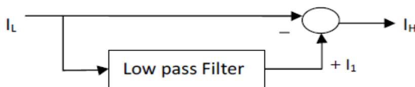
Figure 3.1: Reference harmonics current
