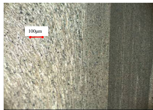
Fig. 12 Microphotograph of aluminum material, welding zone
