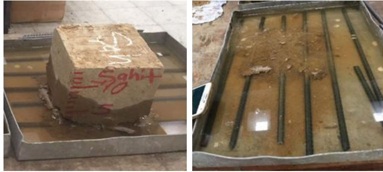
Figure 4. A loss of mass seen with the breakdown of an adobe block under the influence of water.
