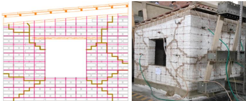
Figure 6. Full-scale adobe model repaired via mud grout injection and reinforced with a \frac{1}{4} " nylon rope mesh. The figure at left shows the repaired cracks and the location of the nylon ropes. The photo at right shows the model on the shaking table before testing.
