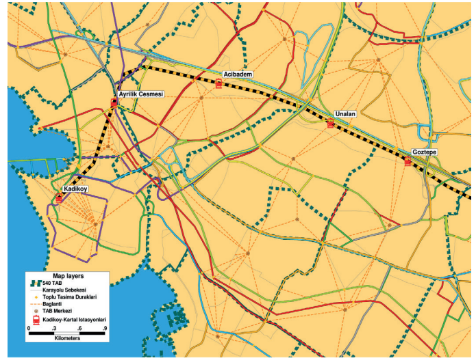
Fig. 5 The model infrastructure of the Kadıköy-Kartal Metro Line between Kadıköy-Göztepe stations in TransCAD: The 540 zones case
