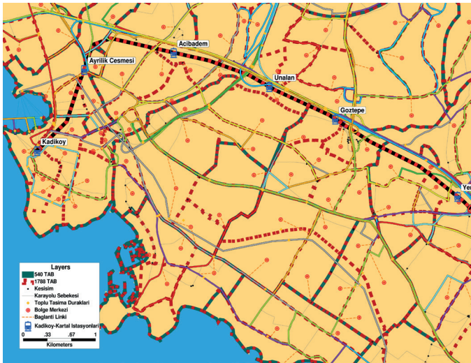
Fig. 8 The model infrastructure of the Kadıköy-Kartal Metro Line between Kadıköy-Göztepe stations in TransCAD : The 1,788 zones case
