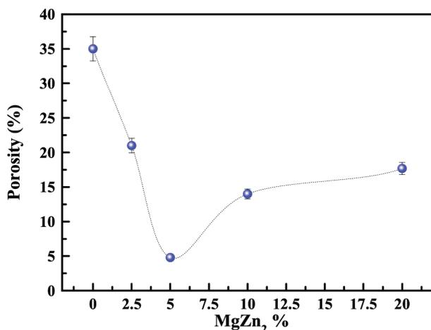
**Figure 2.** Porosity volume fraction of the sintered Al alloy with different  $\text{MgZn}_2$  contents.
