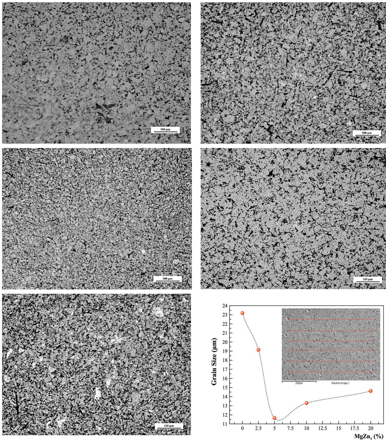
**Figure 3.** Optical micrographs of (a) Al, (b) Al +2.5% MgZn<sub>2</sub>, (c) Al +5% MgZn<sub>2</sub>, (d) Al +10% MgZn<sub>2</sub>, (e) Al +20% MgZn<sub>2</sub>, and (f) grain size measurement.
