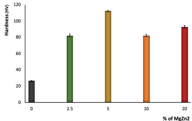
**Figure 6.** Microhardness of Al with different MgZn<sub>2</sub> contents.
