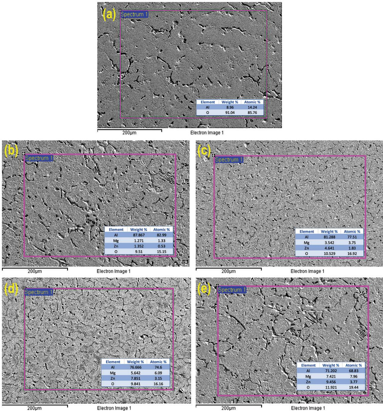
**Figure 4.** SEM surface morphology and EDS analysis of (a) Al, (b) Al + 2.5% MgZn<sub>2</sub>, (c) Al + 5% MgZn<sub>2</sub>, (d) Al + 10% MgZn<sub>2</sub>, (e) Al + 20% MgZn<sub>2</sub> and (f) magnified precipitates formation.
