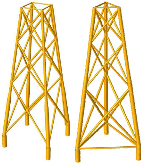
Figure 1. Three-legged and four-legged jacket substructures.
