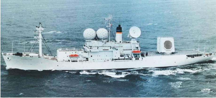
Figure 10 The wideband phased-array Cobra Judy radar on the U.S. Naval ship Observation Island.
