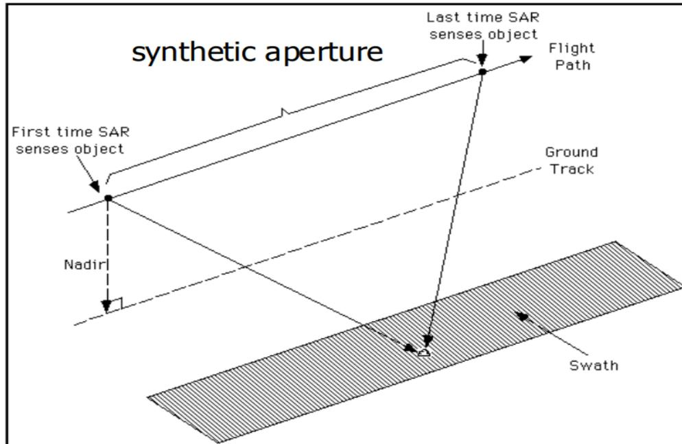
Figure 1. The synthesized antenna by the forward movement of the shuttle.
