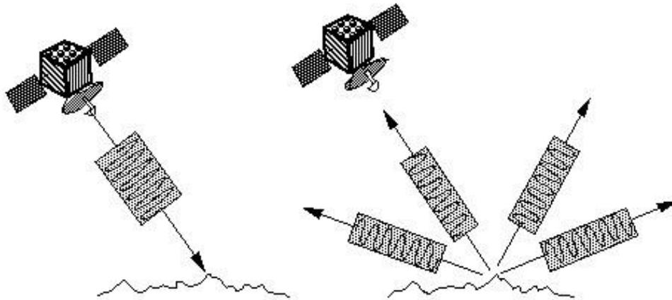
Figure 2. The scattering of radar signal by rough surface.
