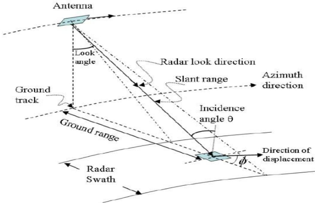
Figure 5. SAR system geometric model.
