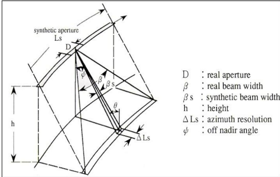
Figure 4. The azimuth resolution of Synthetic aperture radar.
