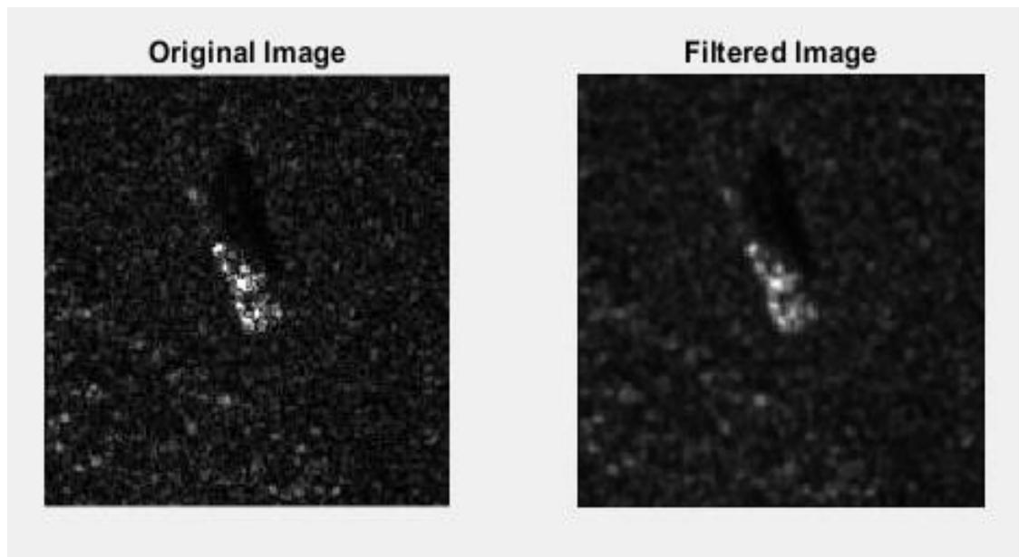
Figure 10. Mean filter applied to SAR image of 2S1 battle tank.
