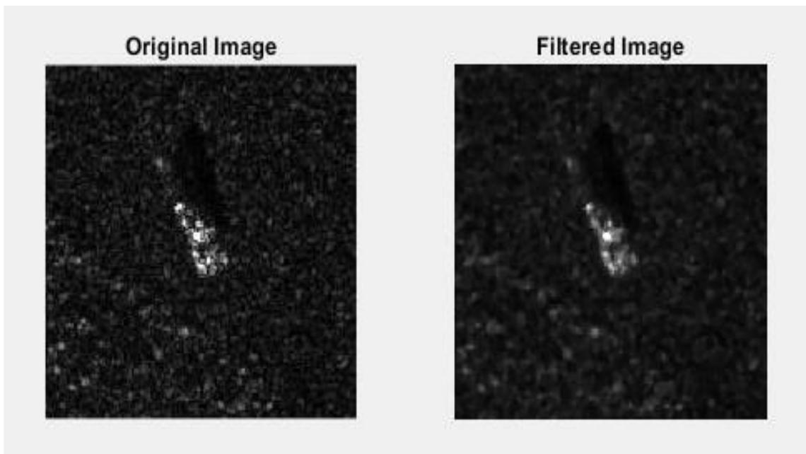
Figure 11. Median filter applied to SAR image of 2S1 battle tank.
