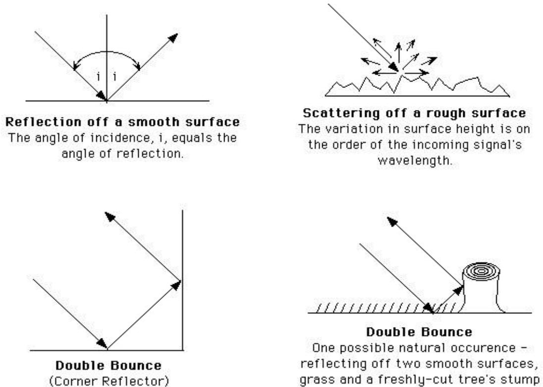
Figure 3. Reflection of radar signals from different types of surfaces.
