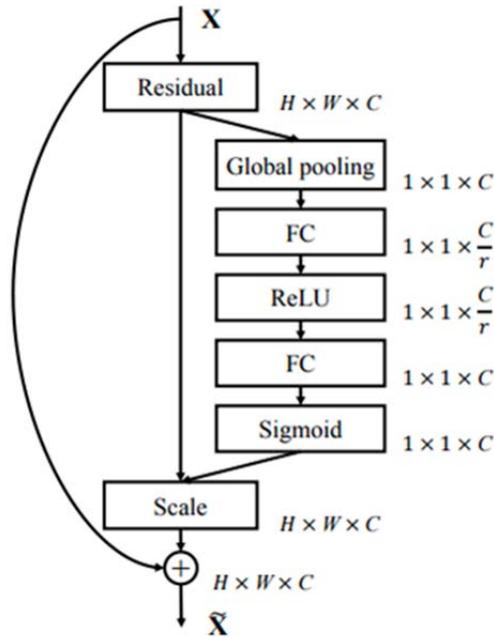
Figure 11 SE-ResNet Architecture.
