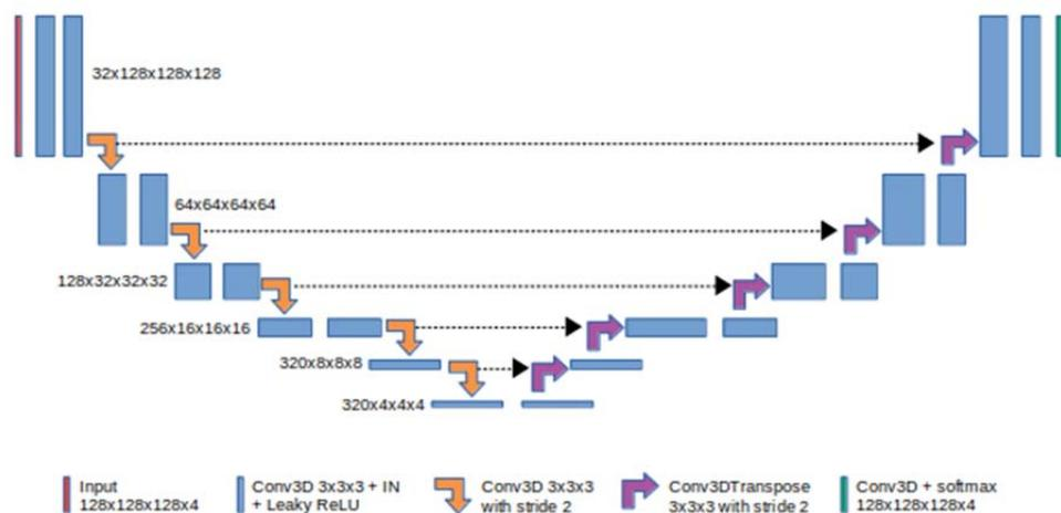
Figure 13 3D U-Net Architecture.
